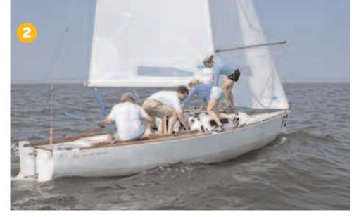
2 As we pass the mark, Jeff keeps the jib trimmed and I ease a lot of mainsheet. This sail trim minimizes weather helm and encourages the boat to bear off smoothly and sharply as we turn downwind. Jo Ann grabs the spinnaker halyard and faces aft (so she can see when and if it's ready to hoist). Meg moves to the cabin top to pre-feed the spinnaker tack from the companionway. Jeff then moves to the cockpit, ready to trim the guy.
