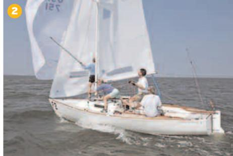
2 Jo Ann releases the pole from the mast, first, then from the guy, and stows the pole. Many foredeck crews prefer the pole jaws up, but Jo Ann prefers to have the jaws down because once the trip line opens the jaws, she pushes the inboard end of the pole down, causing the outboard end to lift away from the guy. I release the weather twing, which allows Meg to hold the guy outboard to keep the spinnaker filled. With the guy in hand, she's ready to drag the spinnaker into the companionway.
