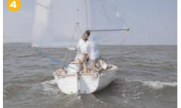
4 The key to the hoist is to get the spinnaker to weather, out from behind the main, where it can fill. Sometimes the pole slides aft as Jeff trims the guy, so Jo Ann will shove the pole forward forcefully while continuing to hoist. Jeff waits to trim the sheet until the guy nearly hits the jaws. Once the spinnaker is clear of the companionway, Meg uncleats the jib halyard and trims the jib sheet so the jib will stay onboard.
